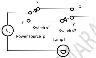
As in the above circuit, two switches S1 and S2 are installed at the bottom and the top of the staircase to operate the lamp L. The lamp turned on by using the switch S1 at the bottom of the staircase can be turned off by using the switch S2 at the top of the staircase. Further, the lamp turned on by using switch S2 at the top of the staircase can also be turned off by the same switch.
